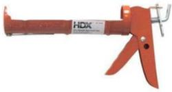
**Caulk Gun:** A tool for pushing caulk out of a tube. It has a trigger grip that advances a rod that goes into the bottom of the caulk tube. Usually \$4.00 to under \$10.00.
